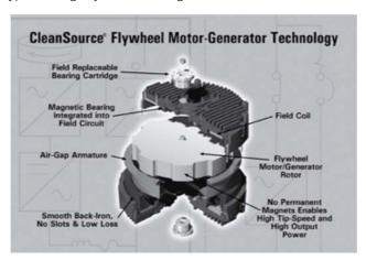
The flywheel rotor is designed to spin in a near frictionless environment by the use of a low-cost combination of a magnetic and mechanical bearing system. The friction in the spinning chamber is further reduced by the creation of a partial vacuum, which reduces the amount of air in the chamber that otherwise creates drag on the
